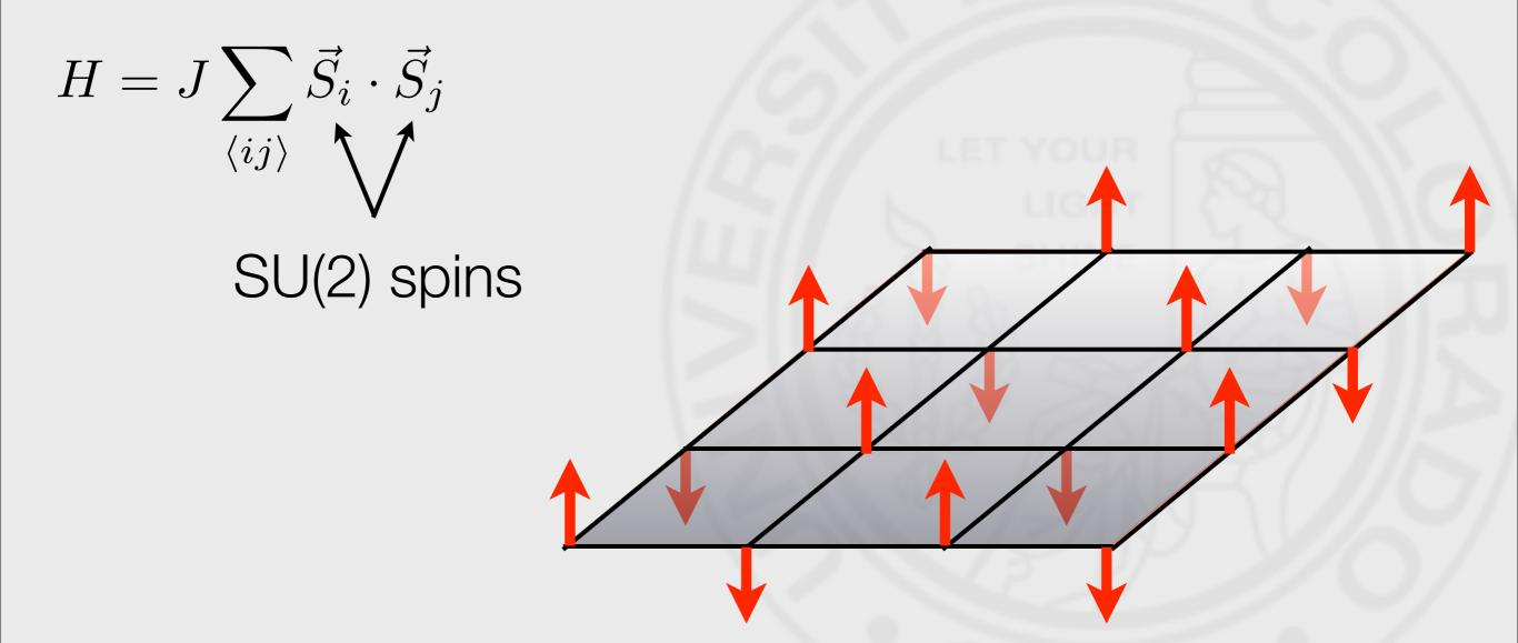
A collection of spin-1/2s on a square lattice in the presence of the antiferromagnetic interactions at T=0 forms a Néel state with a long range antiferromagnetic order (this is known numerically and experimentally).
