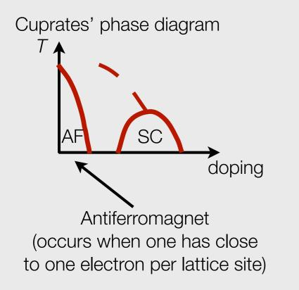
Origin of the antiferromagnetism: Mott insulator of spinful electrons
