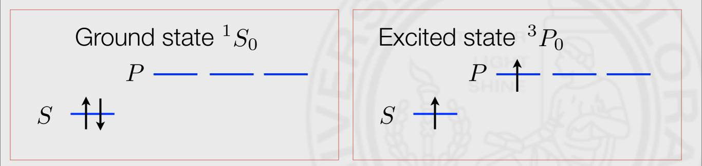
Both of these states have J=0, so the nuclear spin is decoupled from the electronic spin.
